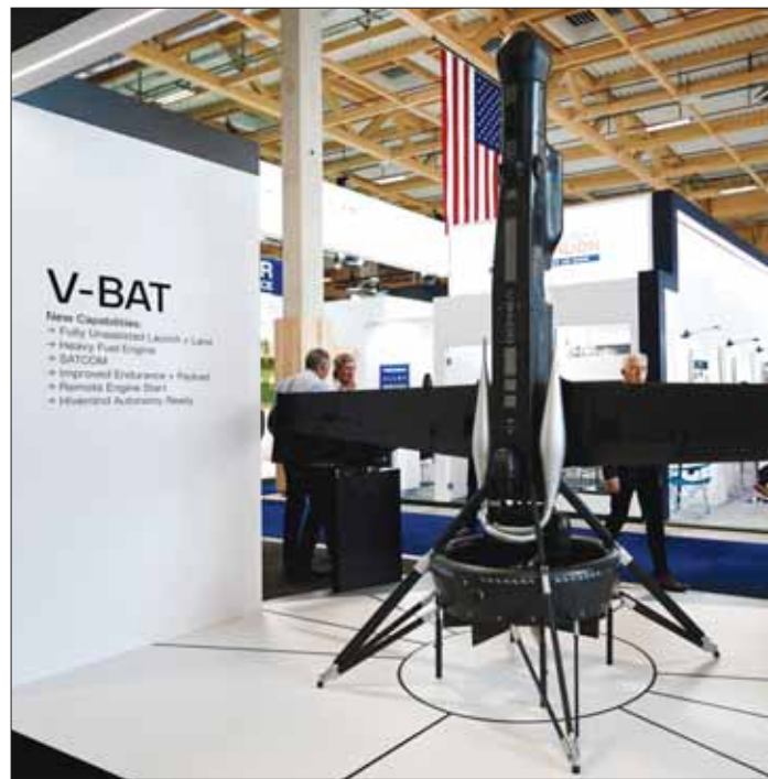
A Shield AI MQ-35 V-BAT vertical take-off and landing unmanned aerial vehicle (UAV) is displayed at the 55th International Paris Airshow at Le Bourget Airport near Paris, France. (Reuters/File Photo)
