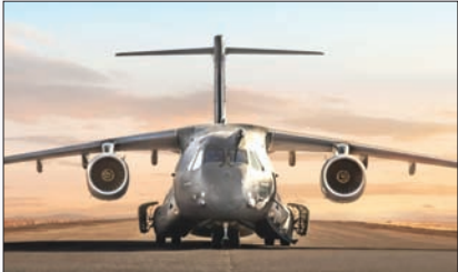
The C-390 Millennium is a multi-mission military transport platform built to carry up to 26 tonnes of payload.
